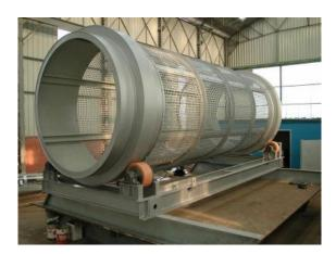
At the end of the sorting process, the waste that is too small (usually less than 7 cm) passes through the meshes and is transferred to the rejected waste. The rest of the waste goes to the vibrating tables to be separated according to their shape.
