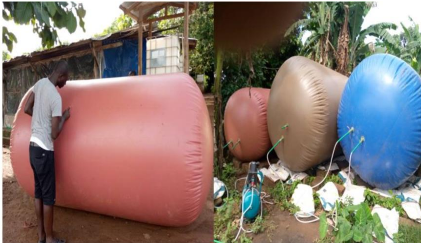
Device for storing filtered biogas in biogas tanks, produced locally by SEFT-AFRICA
